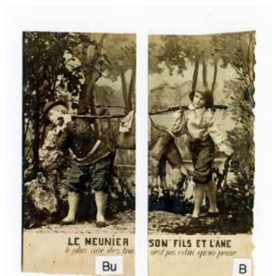
Fig. 8. Image B (right) was exposed to light. Image Bu (left) was the unexposed control.
