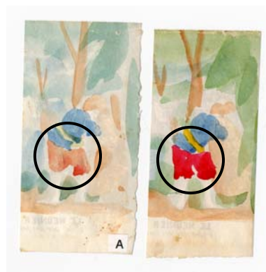
Fig. 10. Image on left shows faded madder red after testing. Image on right is unexposed control.
