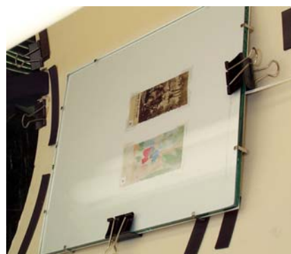
Fig. 2. Samples mounted in light-testing apparatus.
