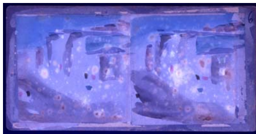
Fig.18. Foxing caused by metabolic products of microorganisms. Fluorescent in UV radiation
