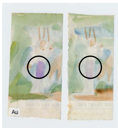
Fig. 12. Image on right shows faded purple color. Image on left is unexposed control.
