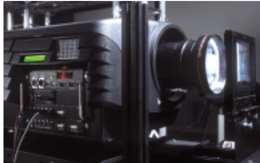
BARCO GALAXY DLP™ An impressive 205 MHz A/D conversion bandwidth ensures compatibility with high resolution and high refresh rate sources for active stereo.
